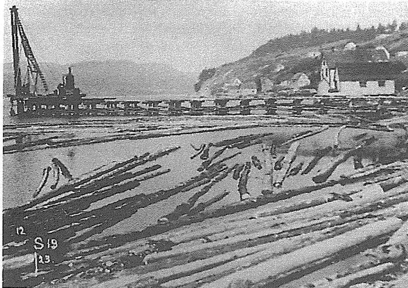
Wood boom at the Fisher sawmill. Doubtless many of the logs were pine like the big tree in the foreground. These pines once grew in abundance on the banks of the Humber. White pine was said to run from 12 to 36 inches in diameter at the butt and up to 40 feet before a limb is reached. The trees grew from 40 to 70 feet tall.
